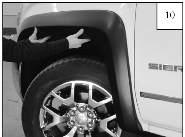
Hold Front Flare up to wheel well to confirm fit. Do not install fasteners at this time.
