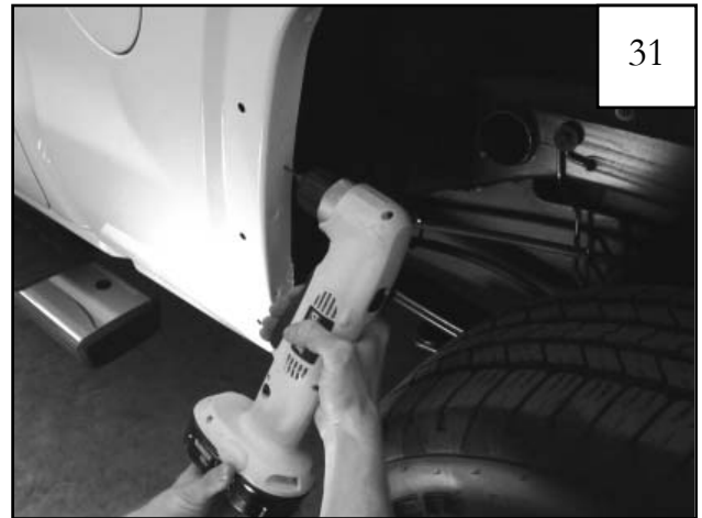
Using a 3/32" drill bit, drill pilot holes through sheet metal at the marks made in Step 30.
